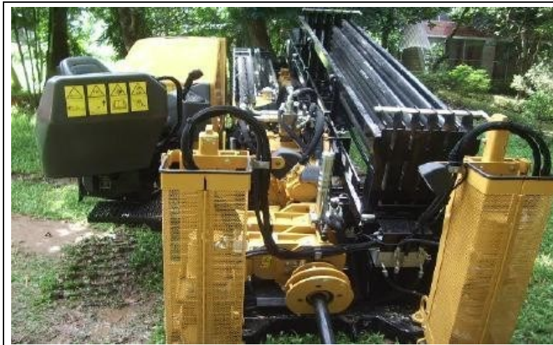
Figure-2.2 Horizontal Directional Drilling (HDD) Machine
